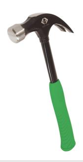
$\sim$  Drop forged high carbon steel head  $\sim$  Hardened & tempered for superior strength and durability  $\sim$  Tubular steel shaft  $\sim$  strong & lightweight  $\sim$  Hi-vis handle for increased visibility in low light conditions  $\sim$  Black lacquered to protect against corrosion  $\sim$  Weight: 568 g / 20 oz Features & Benefits
